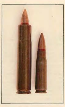
ABOVE: 7.62x62.8mm low-signature cartridge (left) shown in comparison with standard Soviet-manufactured 7.62x39 ball round used in Kalashnikov. Note similarity of case mouth sealants and case lacquers. Photo: Peter G. Kokalis
